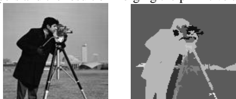
Fig.3.9 The image of cameraman and the result of merging the primitive areas (12 areas remained)
