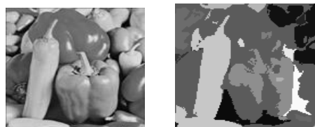
Fig. 3.8 The image of peppers and the result of merging the primitive areas (20 areas remained)
