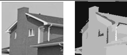
Fig. 3.10 The image of house and the result of merging the primitive areas (20 areas remained)
