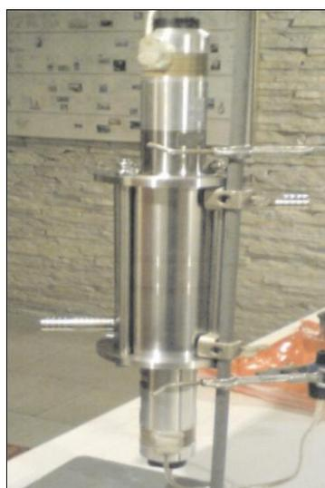
Fig.1. Photo symmetric cavitation reactor on a tripod.
