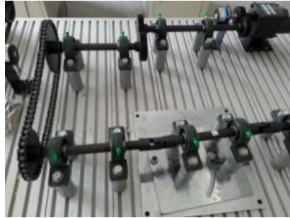
Figure 2 the experiment platform of the transmission system before improving
