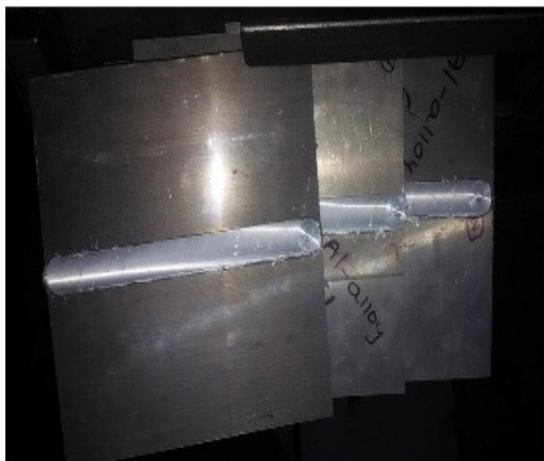
Figure 1 (a) FSW plates; (b) FSW Tool
