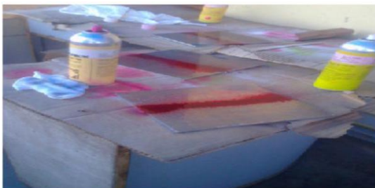
Figure 2 (a) Penetrating test; (b) Ultrasonic test
