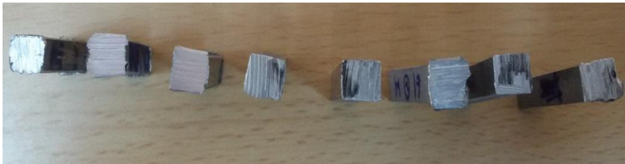
Figure 9 Top view of specimens after wear test
