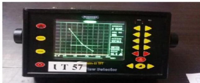
Figure 2 (a) Penetrating test; (b) Ultrasonic test
