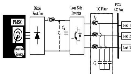
Fig. 1. Standalone wind energy system. Whereas Grid connected system leads to increased energy efficiency, increases support and reliability of system. Due to a relatively low cost of electricity production [2] wind energy is considered to be one of the potential sources of clean energy for the future [3].
