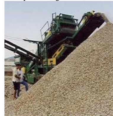
Fig-4 Recycled crushed aggregate of required grading
