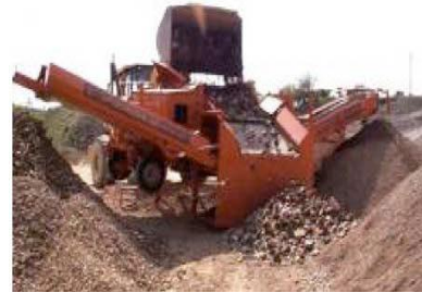
Fig-2 Primary screening removal of soil fraction
