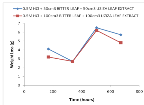
Figure 2: Plots of weight loss against time for Al-1.0wt% Zn immersed in 100cm 3 and 200cm 3 telfaria occidentalis/piper nigrum extract + 0.5M HCl
