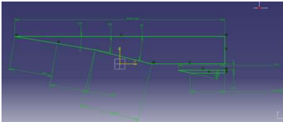
Figure 3: Inlet at mach 8 with 3 ramps(MODEL 3)
