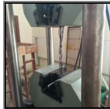
Fig. (3) Testing of prestressing tendons.
