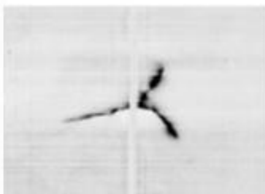
Fig. 2 Microcrack on a solar panel when receiving a Hot Spot
