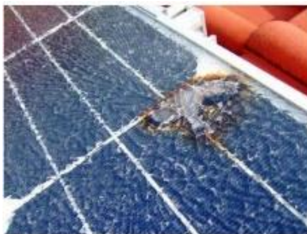
Fig. 3 The solar glass will break when you remove the Hot Spot
