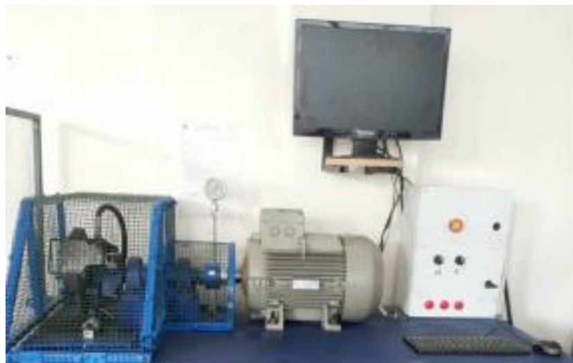
Figure 1. Computer controlled pin-on-disc test device
