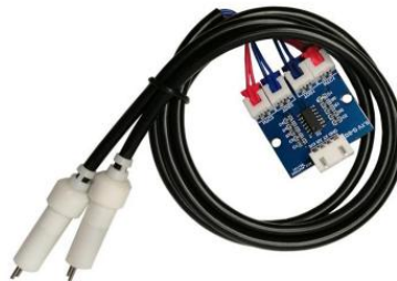
Fig. 4 Dual-channel digital TDS sensor element diagram
