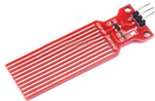
Figure 5 Water level sensor
