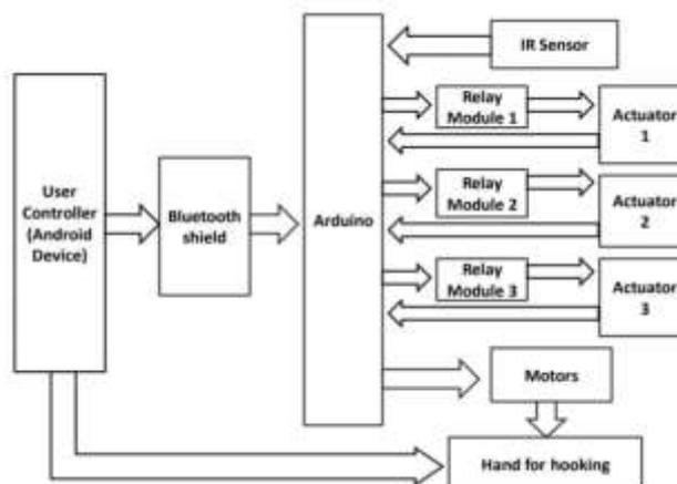
Block Diagram actually how the control circuit has been implemented for EPDRO to serve its purpose. Bluetooth controller is used to give the robot instructions when to start climbing or when to break. As soon as
