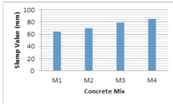
From the above graph the slump value is increased as the percentage of the replacement of coarse aggregate by coconut shell is increased. Therefore, the construction work requiring the more slump value, this type of concrete is suitable. The compressive strength of concrete is detailed in the table below.
