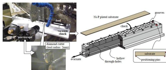
Fig. 2: Diamond shaper-cutting of a thin Ni-P plated substrate using a vacuum chuck.
