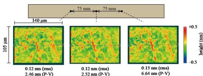
Fig. 6: Roughness of the polished Ni-P plated substrate, measured with white light interferometer (Newview 7200, ZYGO)
