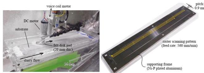
Fig. 4: Polishing of a Ni-P plated substrate in a tilted container with flowing slurry, and the raster scanning pattern of the polishing tool.
