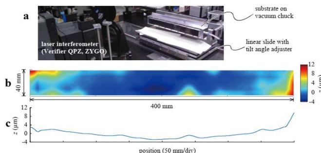
Fig. 5: Form measurement of the Ni-P plated substrate: (a) the measurement setup using laser interferometer, (b) form deviation map and (c) form deviation in cross-section along the centerline.
