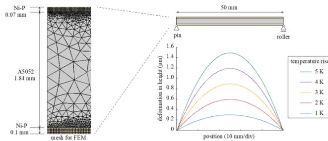
Fig. 3: Simulation result of the bimetallic thermal deformation of a Ni-P plated substrate caused by uneven plating thickness. Finite element method software used is COMSOL Multiphysics.
