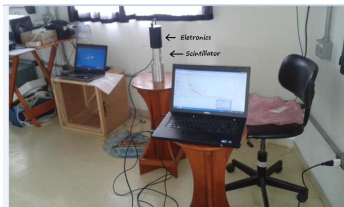
Fig. 1: View of gamma scintillator with associated electronics and computer. (Author)
