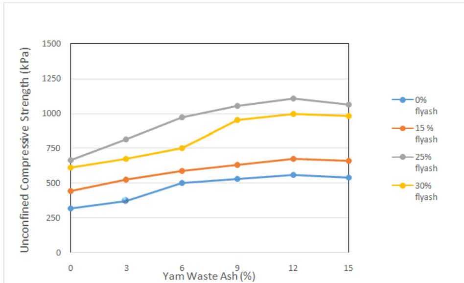
Fig. 1. Influence of Yam Waste Ash on UCS for clay-flyash mixture.
