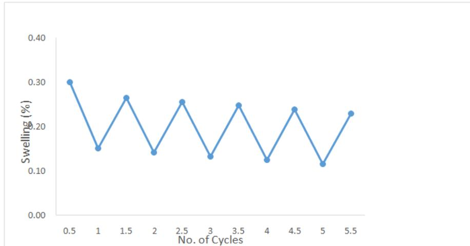
Fig. 4. Influence of number of cycles on swelling of 15% flyash and Yam WA blend under surcharge of 5kPa.
