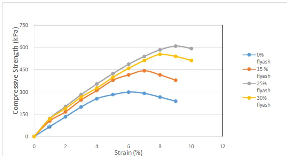
Fig. 2. Influence of flyash on the stress-strain behavior of the soil.
