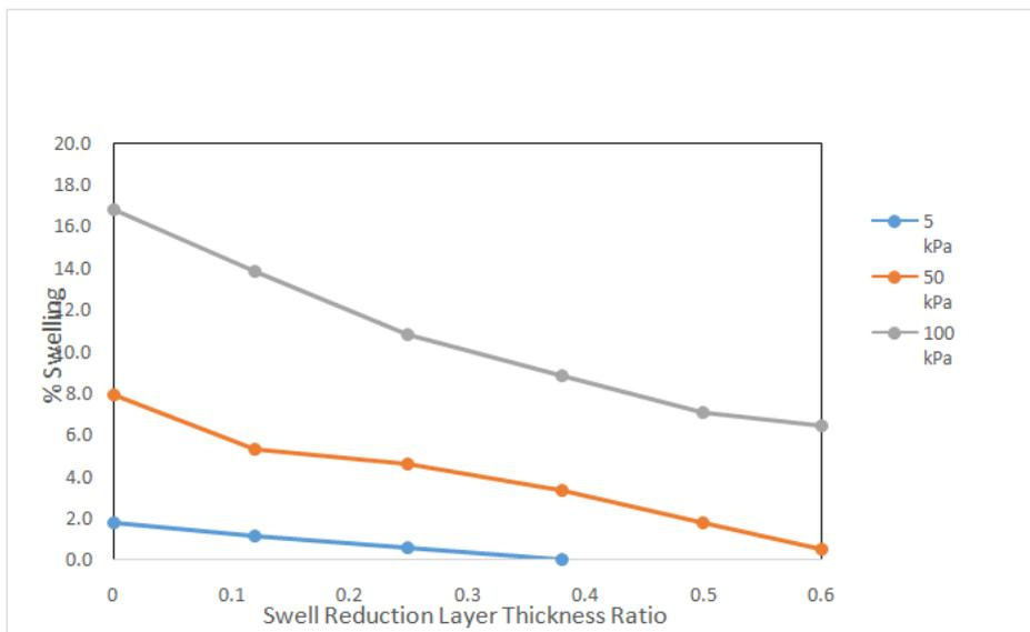
Fig. 5. Influence of Swell reduction layer thickness ratio on swell percentage of soil for various surcharges.
