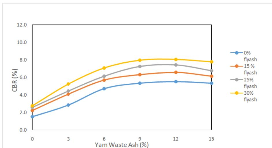
Fig. 3. Influence of Yam Waste Ash on CBR for clay-flyash mixture.
