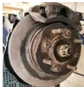
Figure 3. Floating caliper disc brake (FCDB). Figure 4. Main components of FCDB.
