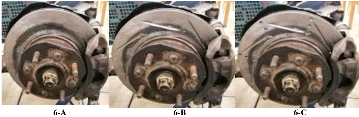
Figure 6. Three different disc brake designs of floating caliper ventilated disc brake system.
