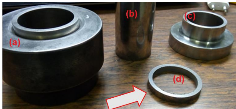
Figure 6: Parts for compacting the specimens in the form of a ring. Thus we have: (a) external matrix; (b) internal matrix; (c) upper puncture; (d) compacted ring
