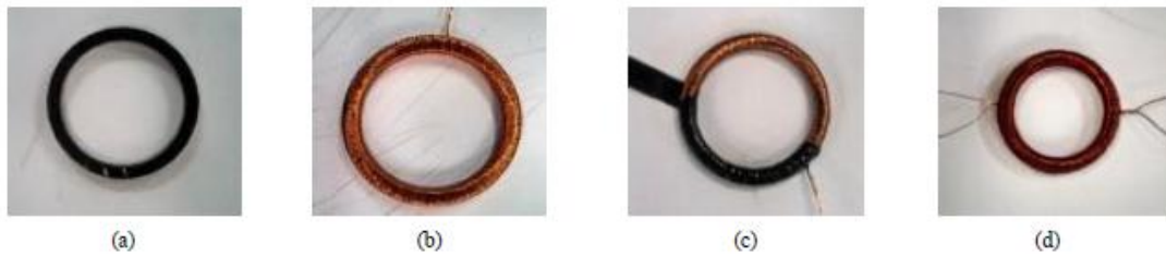
Figure 7: Preparation steps. (a) insulation, (b) secondary winding, (c) insulating and (d) primary winding
