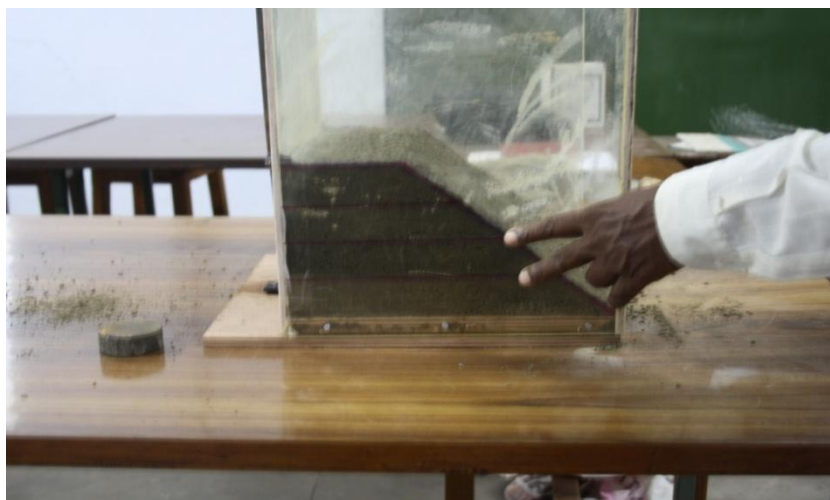
Fig.12 Physical model with two layers of geogrid one at 25% and another at 50% of dump height
