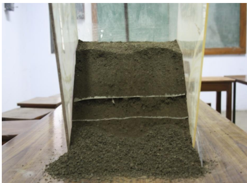
Fig.13 Physical model with two layers of geogrid one at 25% and another at 50% of dump height, at failure
