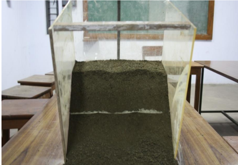
Fig.11 Physical model with one layer of geogrid at 50% of dump height, another view
