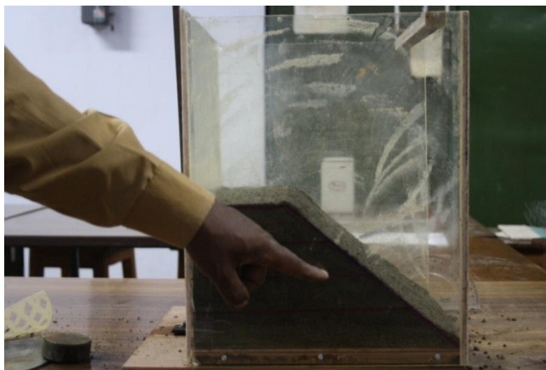
Fig.10 Physical model with one layer of geogrid at 50% of dump height
