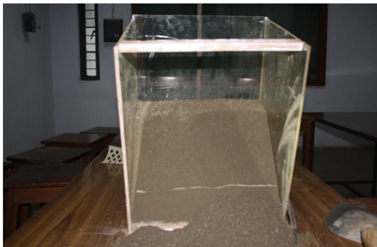
Fig.9 model with one layer of geogrid at 25% of dump height another view
