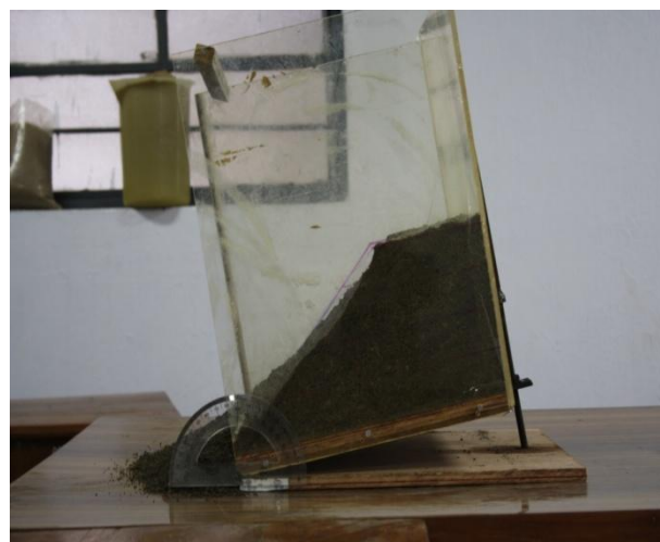
Fig.7 Basic Model without any geogrid at failure
