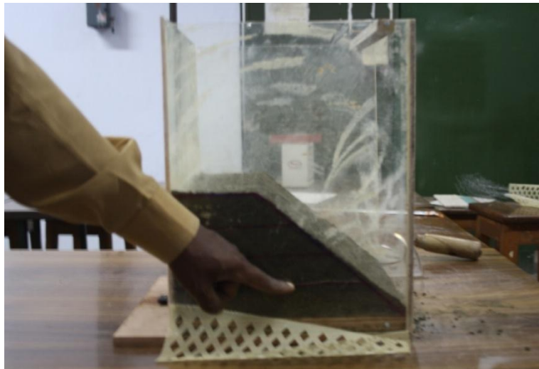
Fig.8 model with one layer of geogrid at 25% of dump height
