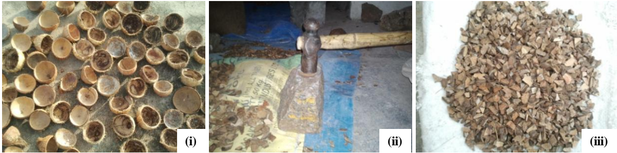
Figure 1 Processing of coconut shells: (i) air drying at 25-30°C, (ii) breaking coconut shells and (iii) sieved coconut shells through 12mm sieve.
