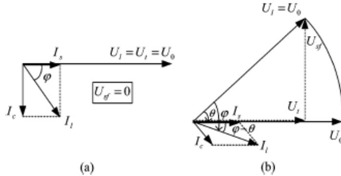
Fig. 4. Phasor diagram of quadrature compensation. (a) Without voltage sag.
