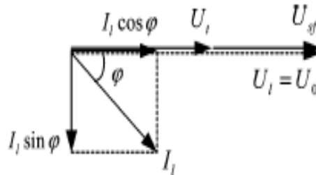
Fig. 5. Phasor diagram of inphase compensation (supply voltage sag).
