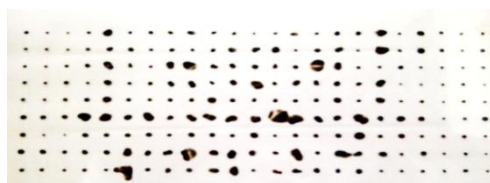
Figure 9. Ink pattern after force application over the tire. Only some of the points of the pattern are deformed, these points are in contact with the surface and the tire.
