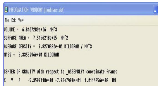
Figure 12. Weight and C. G. of fixture in Quadrant III
