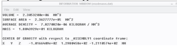
Figure 24. Weight and C. G. of fixture in Quadrant I
