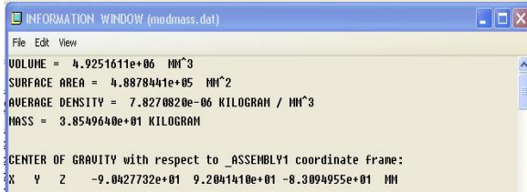
Figure 10. Weight and C. G. of fixture in Quadrant I
