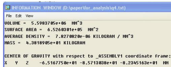
Figure 13. Weight and C. G. of fixture in Quadrant IV
