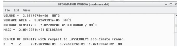
Figure 31. Weight and C. G. of fixture in Quadrant VIII
