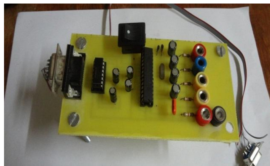
Fig. 7 Map of universal asynchronous serial interface built around the 16F876A microcontroller.
