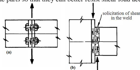
Figure 1 - Strain to shearing joints (a) screwed and (b) welded
