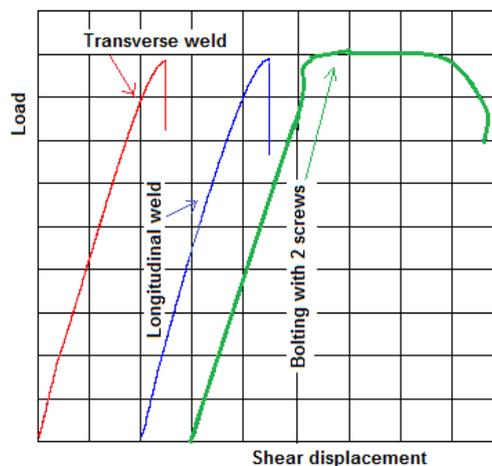
**Figure 8** - Load curve as a function of displacement for welded joints and bolts joints
