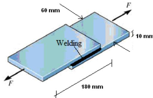
Figure 3 - Welded plates for shear test
