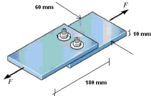
Figure 2 - Plates bolted to the shear test
