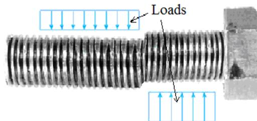
**Figure 5** - Crushing shear bolt due effort
