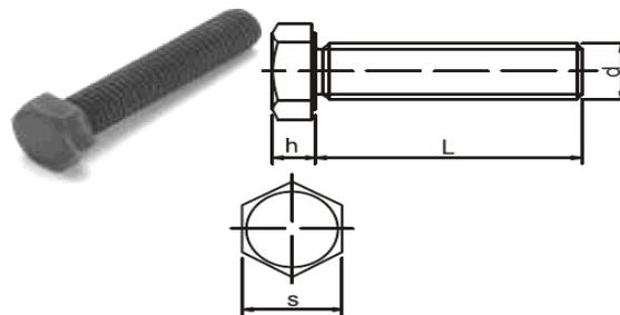
Figure 4 - Hex fixing screws
