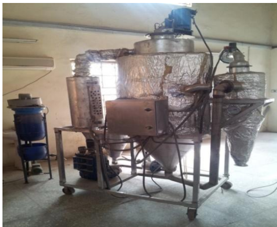
Figure 4: Spray Dryer Developed at the Hydraulic Equipment Development Institute (HEDI), Kano, Nigeria
