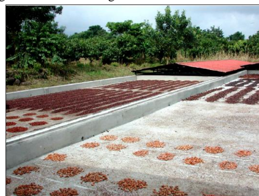
Diagram 5: Showing actual mobile roof solar cocoa dryer used in Venezuela, Taken from Sukha 2009
