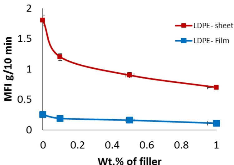
Figure 3. Melt flow index for LDPE films, sheets and their nanocomposites
