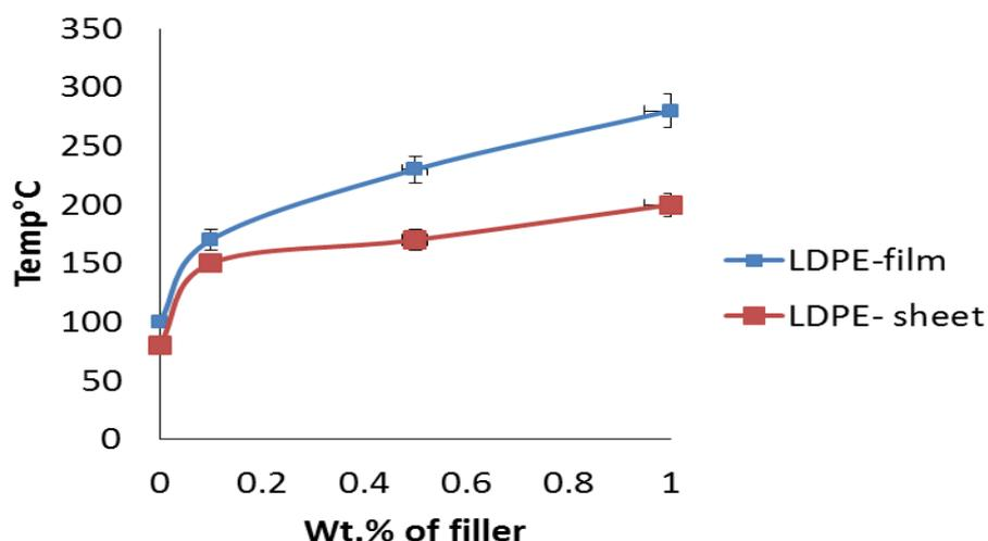
Figure 4. Temperature versus Wt. % of nanofiller for LDPE
