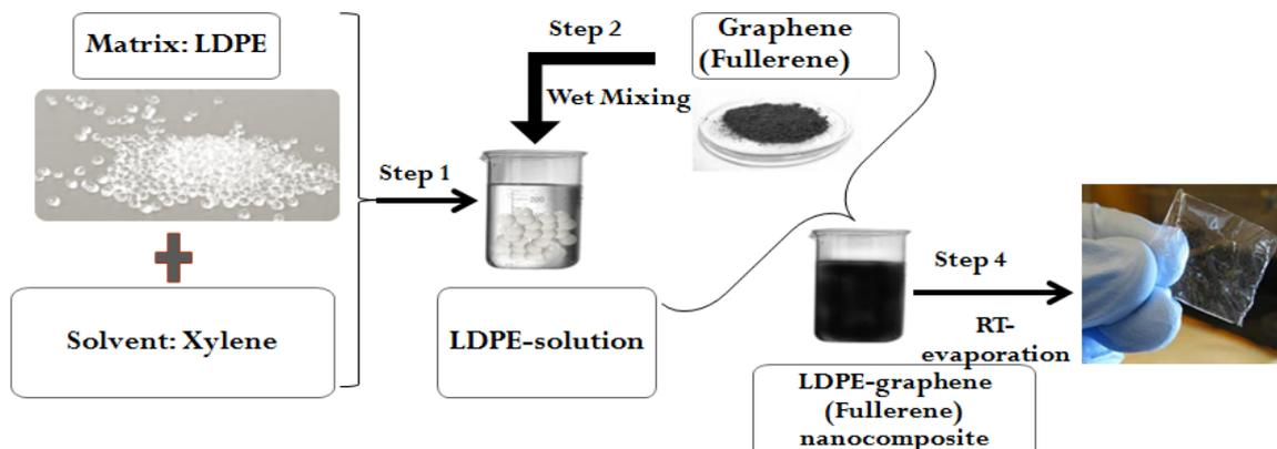
Figure 1. Fabrication of LDPE Membrane
