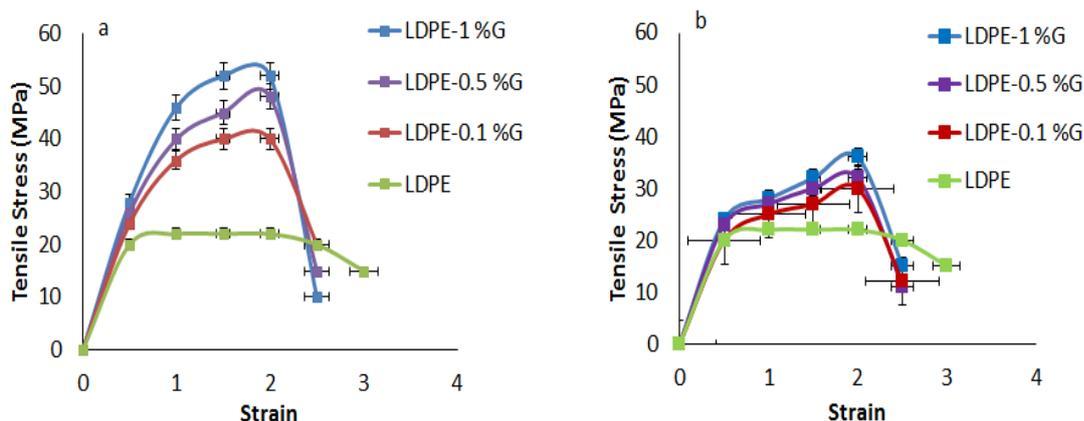
Figure 2. Stress-strain curve for LDPE and LDPE nanocomposite membranes a) LDPE thin film b) LDPE sheet
