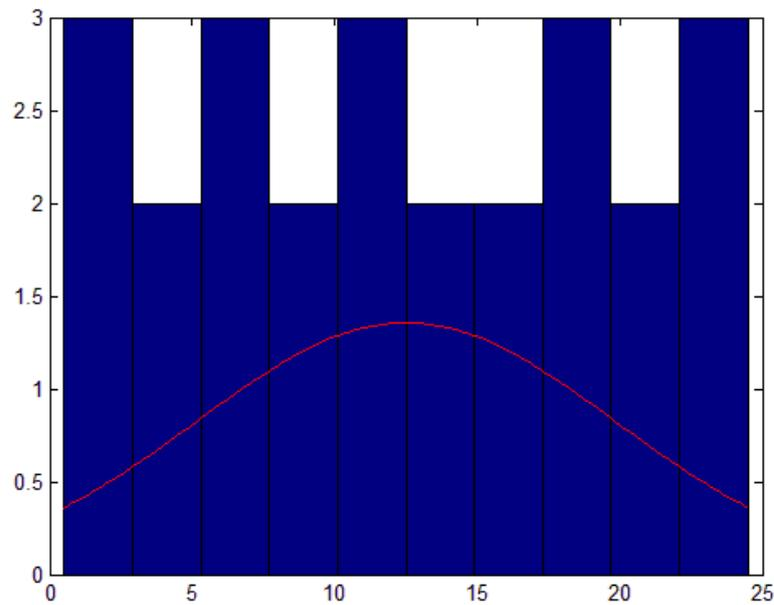
According to the statistical analysis of the observed data, the speed of the ship in the course of the passage obeys normal distribution , in which, the mean value is 12.5kn (converted to23.0km/h for convenient calculation)and the variance is 2.
