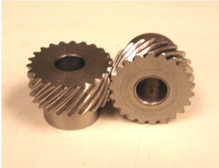
Figure 9. A Helical Gear Set Made with a Standard Tap
