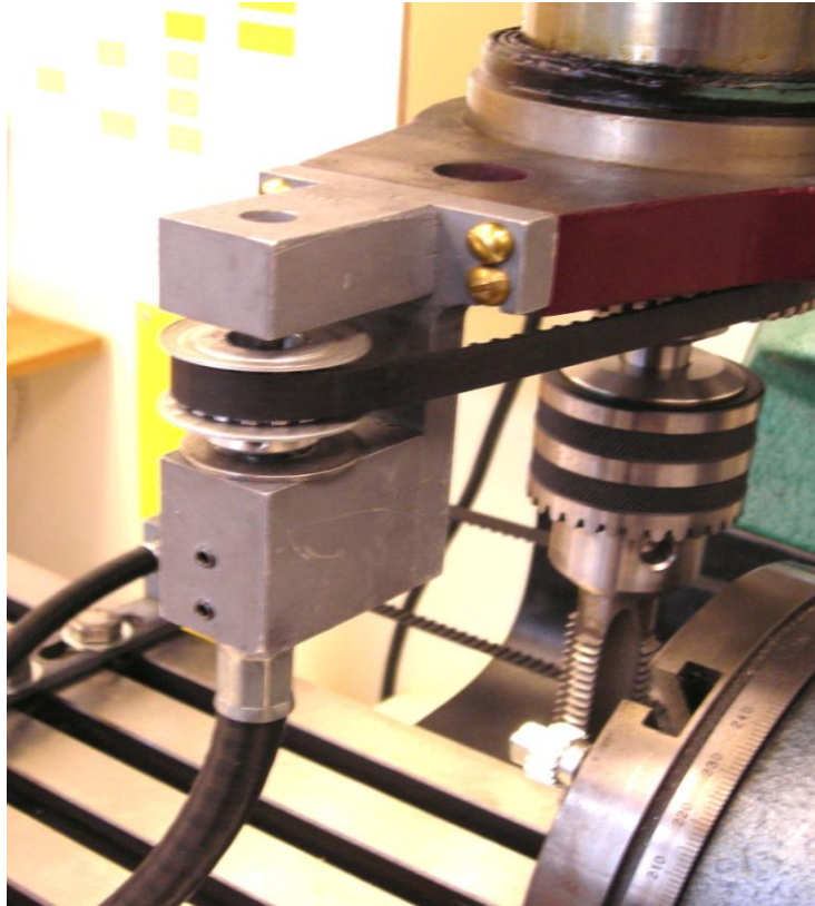
Figure 3. Vertical Fixture for First End of Flexible Shaft
