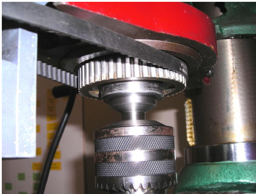
Figure 2. Drive Pulley Fixed to Mill Spindle
