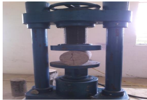
Fig. 6 Split Tensile Strength Test
