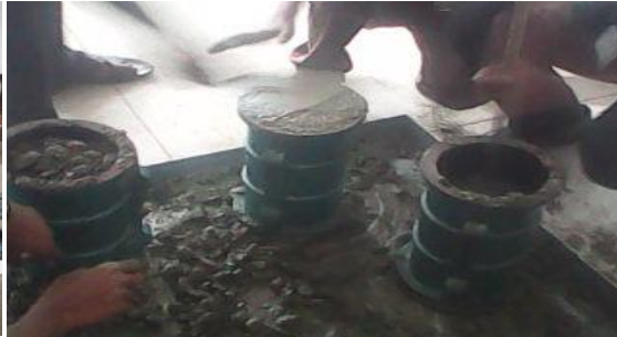
Fig.3 Casting of Test Specimens
