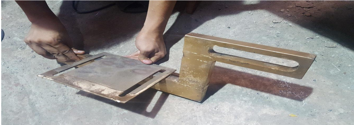
Figure 4 shows Base plate and Frame used in the attachment
