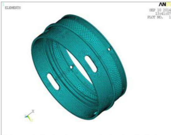
Figure 5: Finite Element Meshed Model of the Bulk Head Support Component
