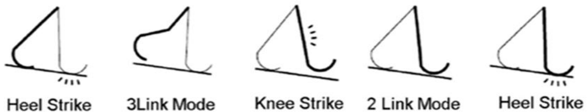
Fig 7: Leg movement of Prosthetic Limb
