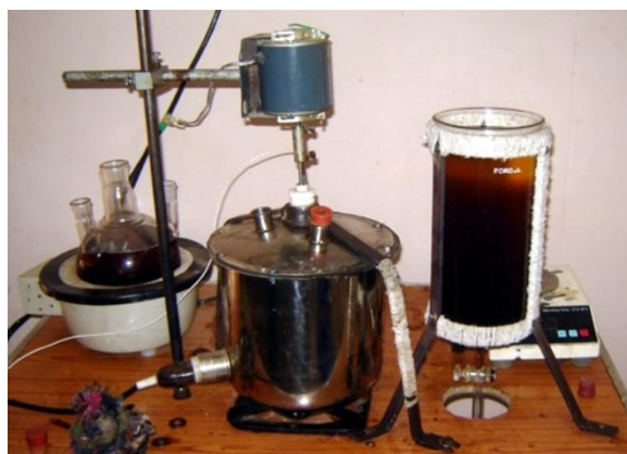
Figure 1 Photographic view of Biodiesel preparation plant (transesterification process)
