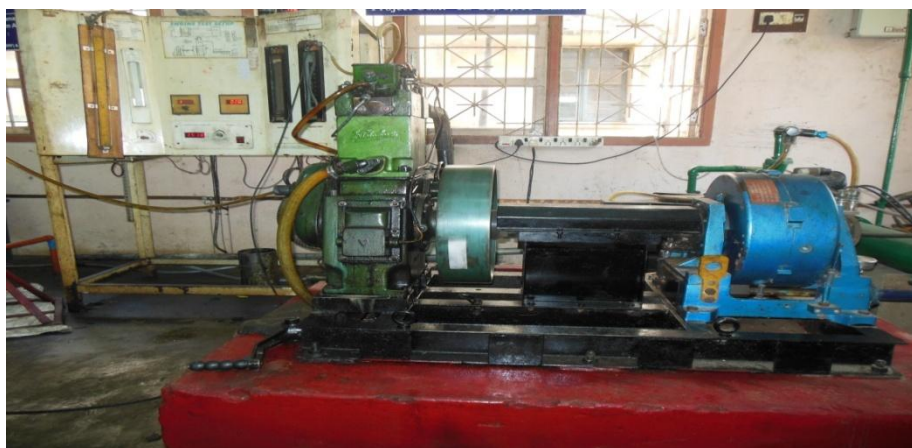
Figure 2. Four stroke engine with eddy current dynamometer test rig
