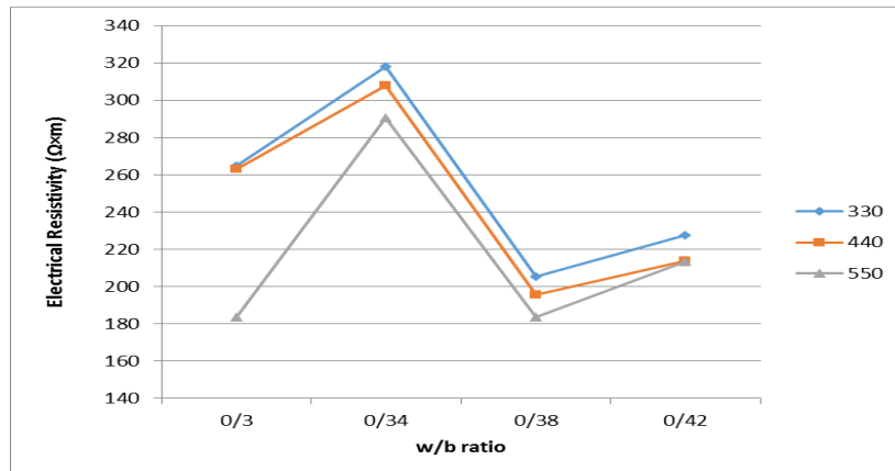
Fig. 8 - Results of electrical resistivity test in different w/b ratios and binder contents
