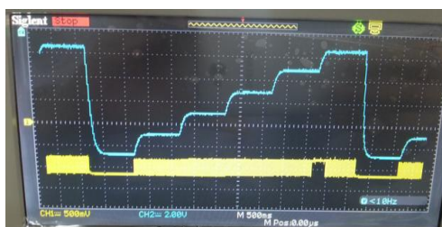
Figure 7 Stepped output of PWM waveform forming of PWM circulation regulation
