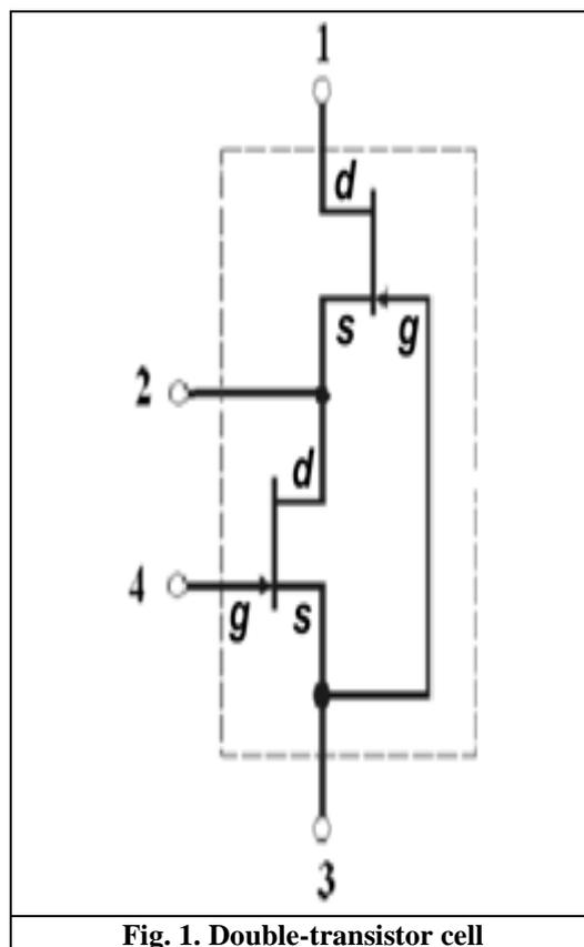
Creating a common contact to the source and gate regions of the primary transistor reduces the series resistance of the source and gate regions, excluding the input signal loss. This opens the possibility of its use as a stabilized current generator. Pinch-off voltage of the primary field-effect transistor is 0.8 V with a negative temperature coefficient and in additional field-effect transistor is 0.5 V - with a positive coefficient that provides a thermally stable mode, fig. 2.
