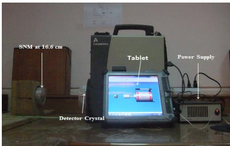
Fig.(2). Experimental setup arrangement for activity measurement without collimator
