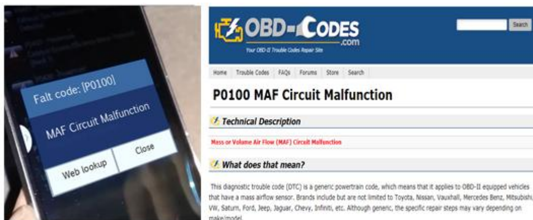
Figure 7. Identification and illustration of the fault code using the Internet.
