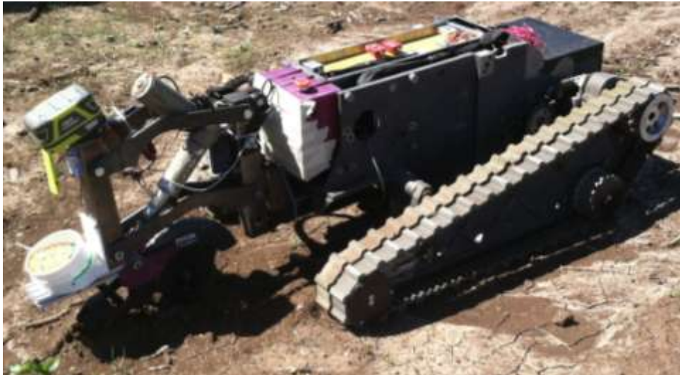
Figure 1: KSU- BAE UGV with a prototype planter sowing wheat seed.
