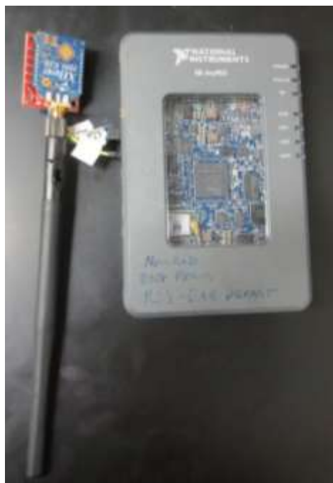
Figure 2: NI myRIO 1900 with XBee Pro S3B antenna
