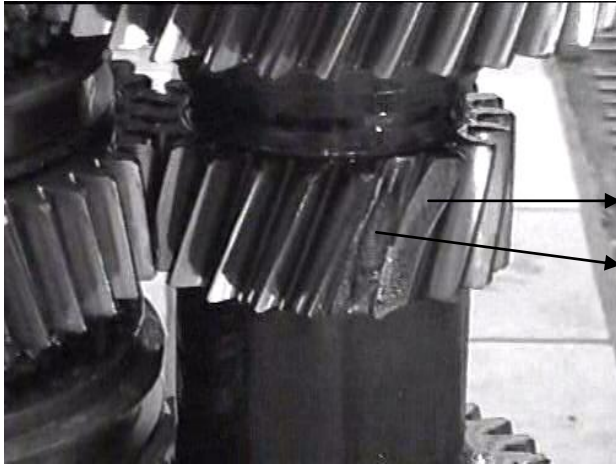
View of spindle shaft gearing and marking of damages:
