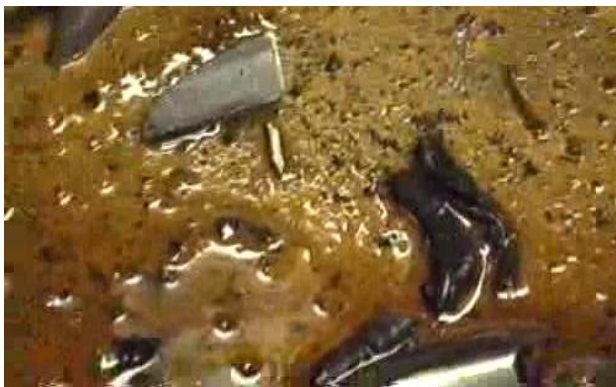
View of fragments found in the gearbox
