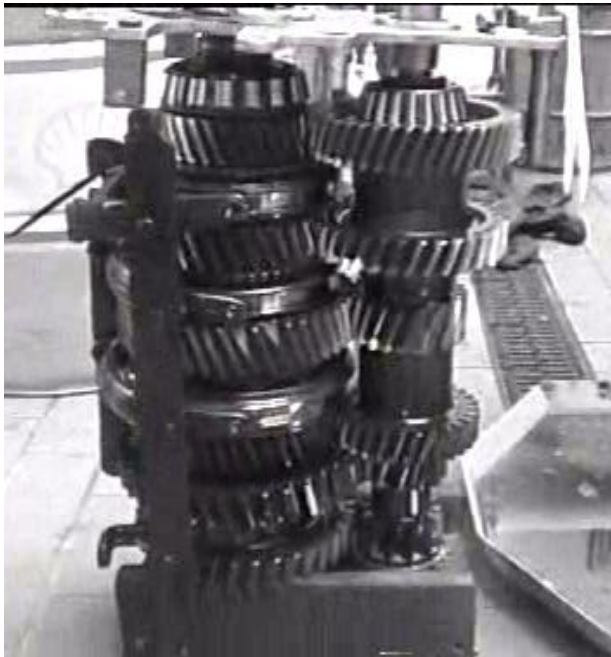
view of the spindle gear shaft after removal from the gearbox housing
