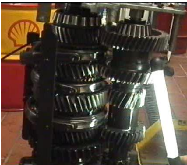
a closer look at the gear shafts with gear wheels
