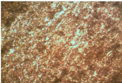
**Figure 10:** micrograph of Al-Si alloy-10wt % SiC composite
