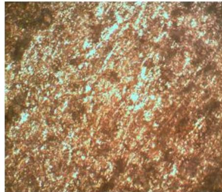
**Figure 9:** micrograph of Al-Si alloy-5wt % SiC composite
