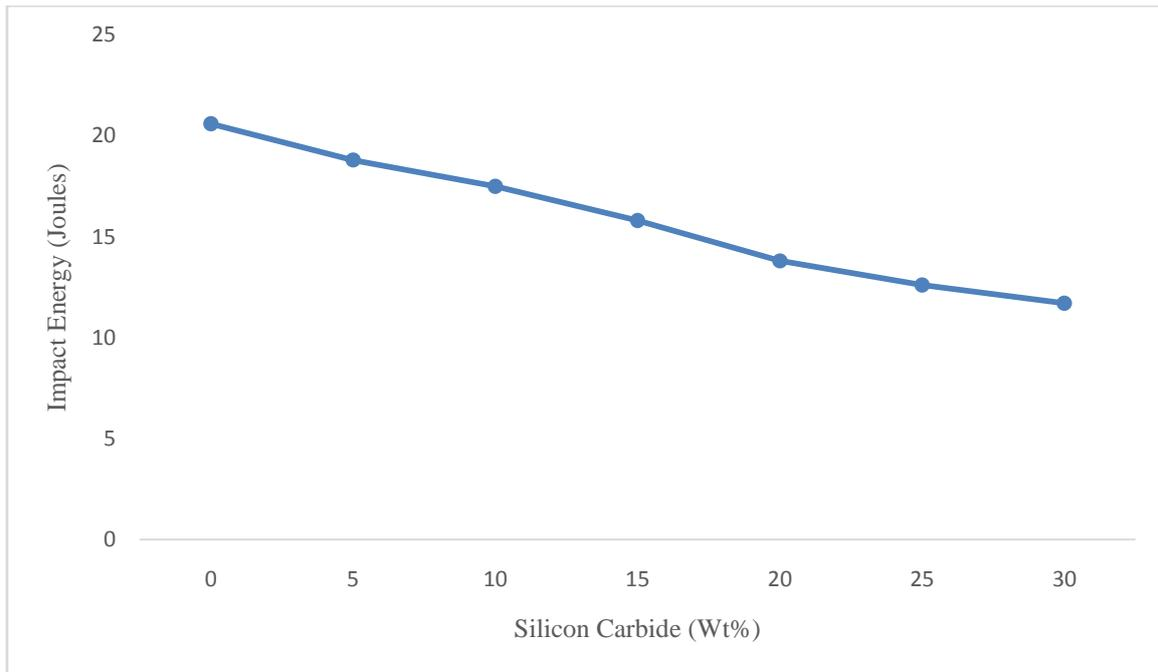
**Figure 6:** effect of silicon carbide addition on impact on energy of Al-Si alloy
