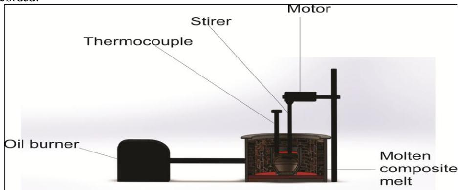
**Figure 1:** Diagram showing the stir casting set up
