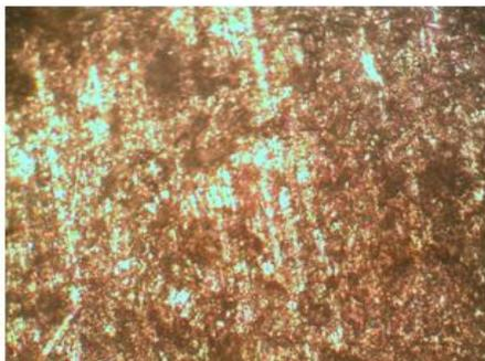
**Figure 12:** micrograph of Al-Si alloy-20wt % SiC composite
