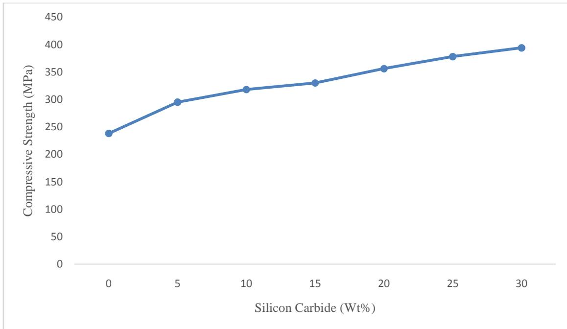
**Figure 4:** effect of silicon carbide on compressive strength (MPa) of Al-Si alloy
