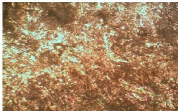
**Figure 14:** micrograph of Al-Si alloy-30wt % SiC composite
