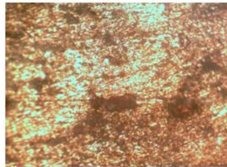
**Figure 11:** micrograph of Al-Si alloy-15wt % SiC composite
