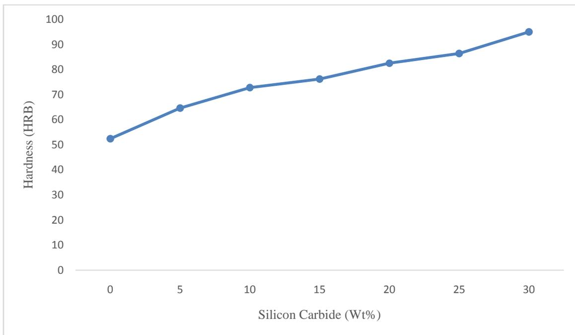
**Figure 5:** effect of silicon carbide addition on hardness of Al-Si alloy
