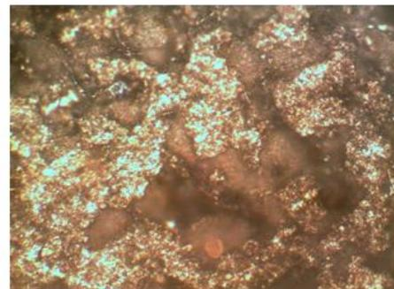
**Figure 13:** micrograph of Al-Si alloy-25wt % SiC composite
