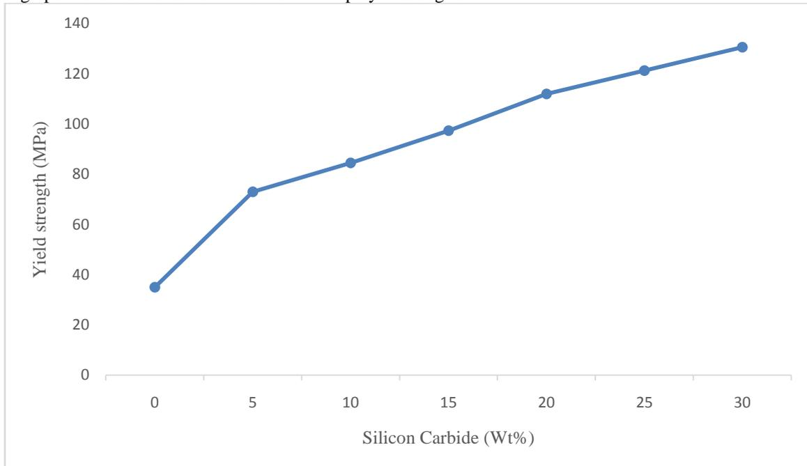
**Figure 2:** effect of silicon carbide addition on yield strength of Al-Si alloy
