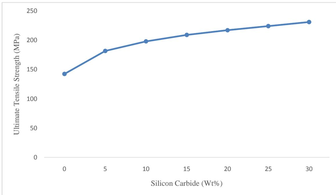
**Figure 3:** effect of silicon carbide addition on ultimate tensile strength (MPa) of Al-Si alloy
