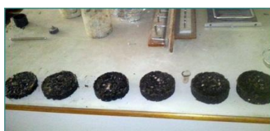
Fig 2:- Premix Carpets with different thickness or height to find out the required quantity of materials to produce 20 mm thick Premix Carpet.
