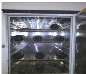
Fig. 8 : premix carpets, coarse aggregates and slurry seal type II mixed together
