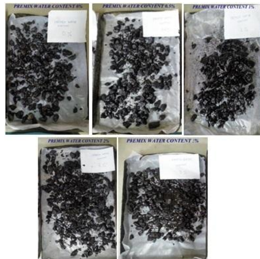
Fig 1: Coating Test with 0%, 0.5%, 1%, 2%, 3% pre-mix water by weight of dry aggregate.
