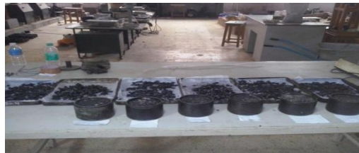
Fig. 3 :- Six different samples with different binder quantity to find out optimum emulsion content
