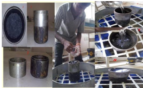
Fig 9: Photographs of conducted permeability test of different premix carpet samples
