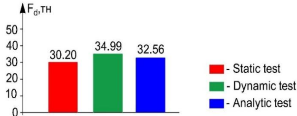
Fig 9. Diagram for comparing the average bearing capacity with a length of 7.0 m.
