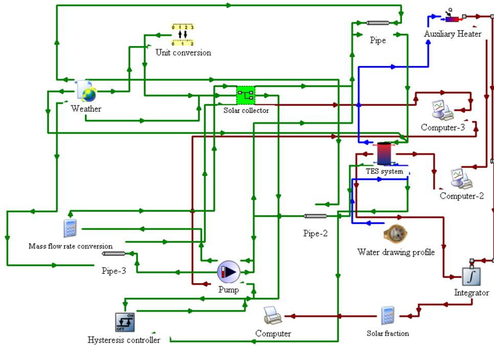
Flow diagram of SWH system (a) for charging cycle (b) without controller (c) with variable controller (d) with hysteresis controller
