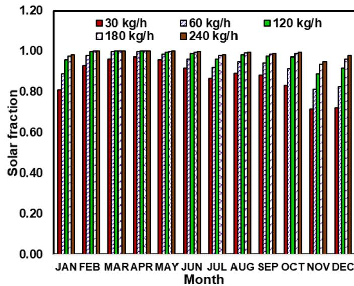
Solar fraction at different mass flow rates of HTF.
