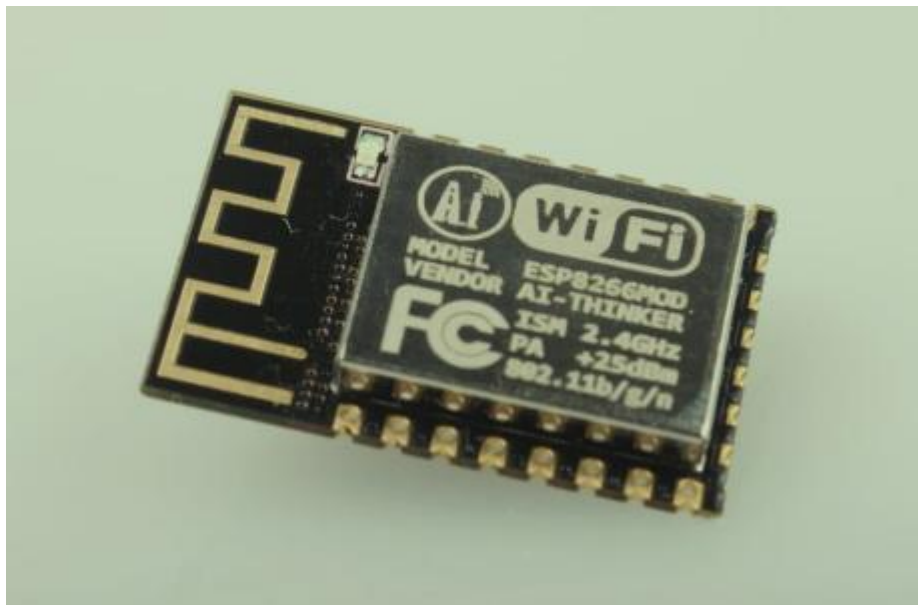
Figure 3 Wi-Fi module ESP8266
