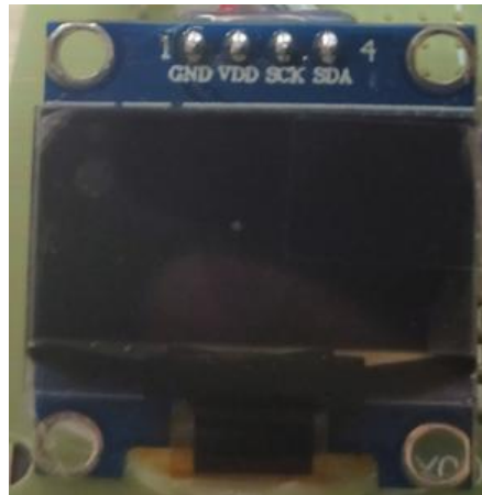
Fig.8 Physical map of OLED12864 display
